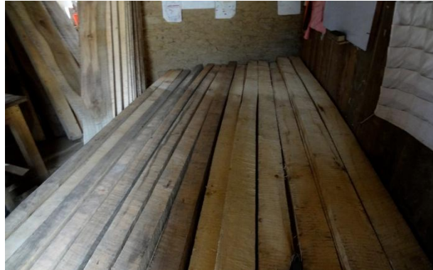
Wood for building being dried
